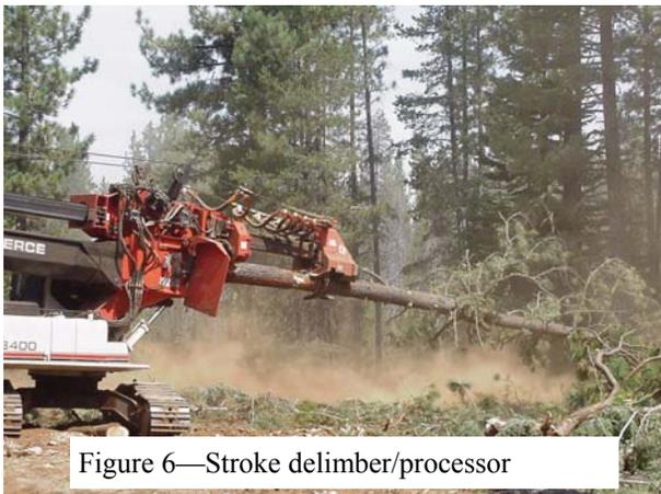
Figure 6—Stroke delimiting processor
