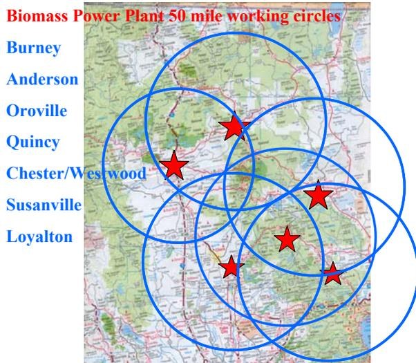
Figure 2—N. California biomass powerplant distribution and fuel supply areas
